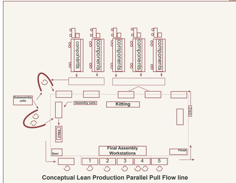
parallel pull flow line. First, workers must be capable of performing all line tasks, a portable assembly worksite is necessary to transport all fixtures along with a complete set of assembly components. All of the necessary tools and a complete kit of parts must be available to each worker at each station. Finally, the assembly procedures must be followed exactly.
